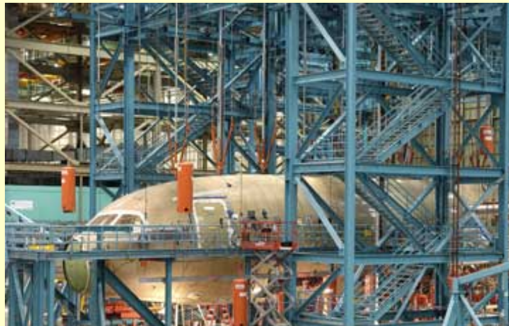
The 787 Dreamliner, shown here in full-scale airframe hydraulic stress testing, is the result of open innovation efforts by Boeing and other companies in the U.S., U.K., Japan, China, and elsewhere.
